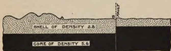
FIG. 109.—Diagram to illustrate some causes of the abnormal values in the local acceleration of gravity. A , A point upon the surface where gravity is strongly influenced by neighboring mountains. B , A point where gravity is affected by the elevation along a fault of a portion of the dense core of the earth.
